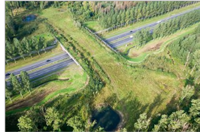
Figure 10. ‘Eco-aqueduct’ over ‘sunken’ motorway on the new A4 in Holland (Google)
